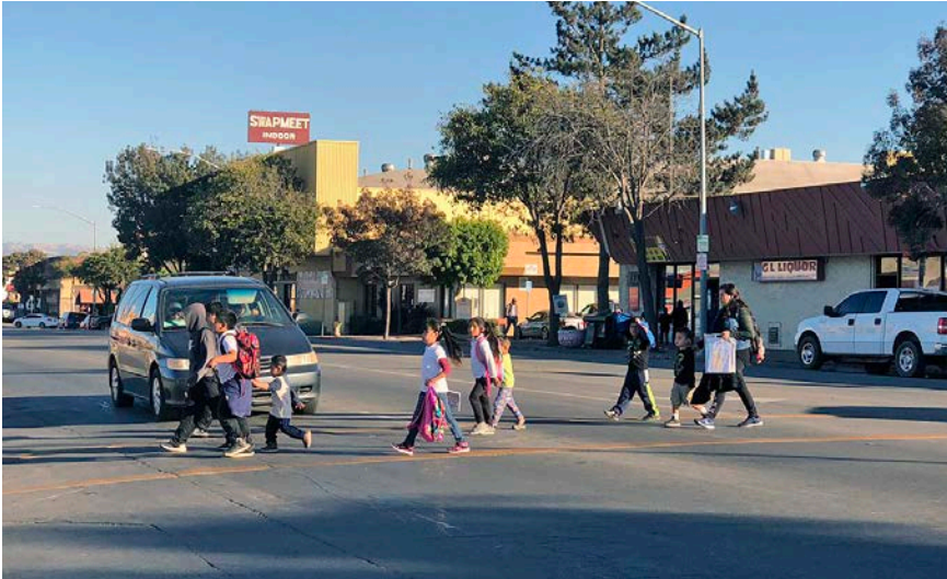
Many pedestrian crossings consist of standard transverse-style crosswalks lacking high-visibility markings.
