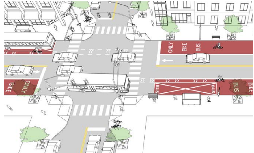
Bus stops located at the far side of intersections can reduce delays for buses and support traffic signal prioritization for transit.
