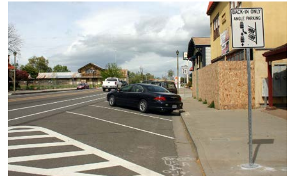
Back-in diagonal parking increases parking capacity and has safety benefits over head-in diagonal parking.
