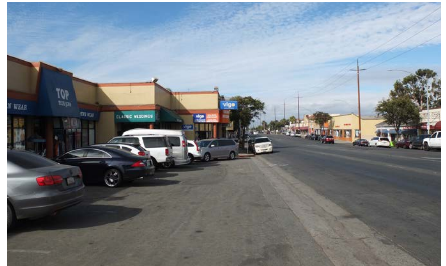
Perpendicular off-street parking exists at several locations along East Alisal Street, leading to potential areas of conflict between motorists and pedestrians.
