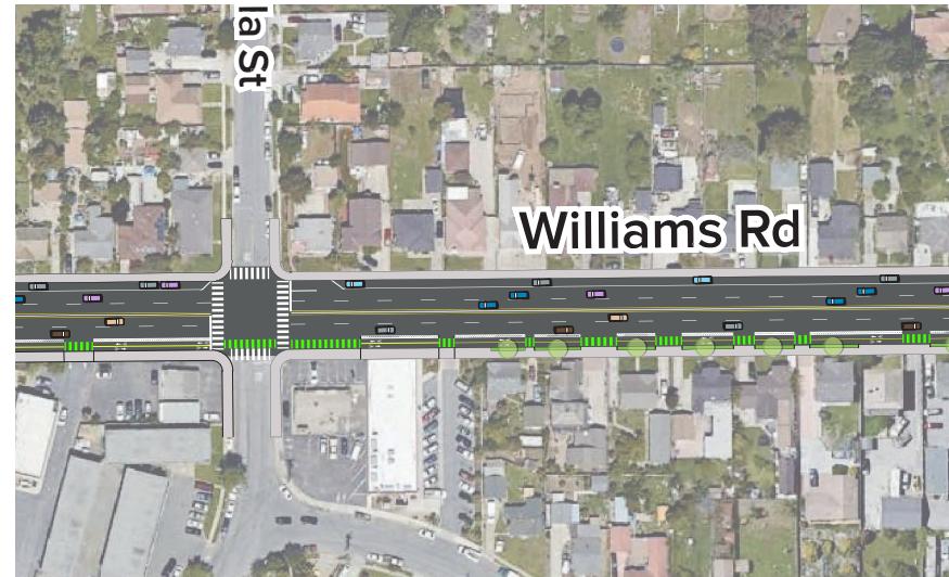
The concept for Williams Road improvements east of the East Alisal Street intersection includes a two-way protected bike lane and enhanced crossings.
