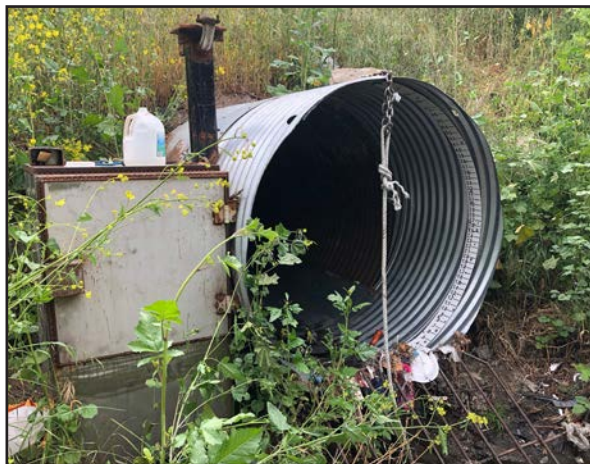
Acosta Plaza terminal outfall structure shown with attached passive sampling water quality equipment (left) used for continuous monitoring of hydrology and pollutant loads (photo taken 5/1/18).
